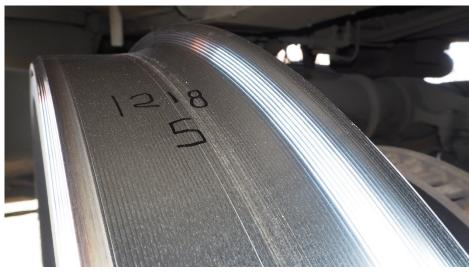
FIGURE 67: APPEARANCE OF REPROFILED VLOCITY WHEEL
