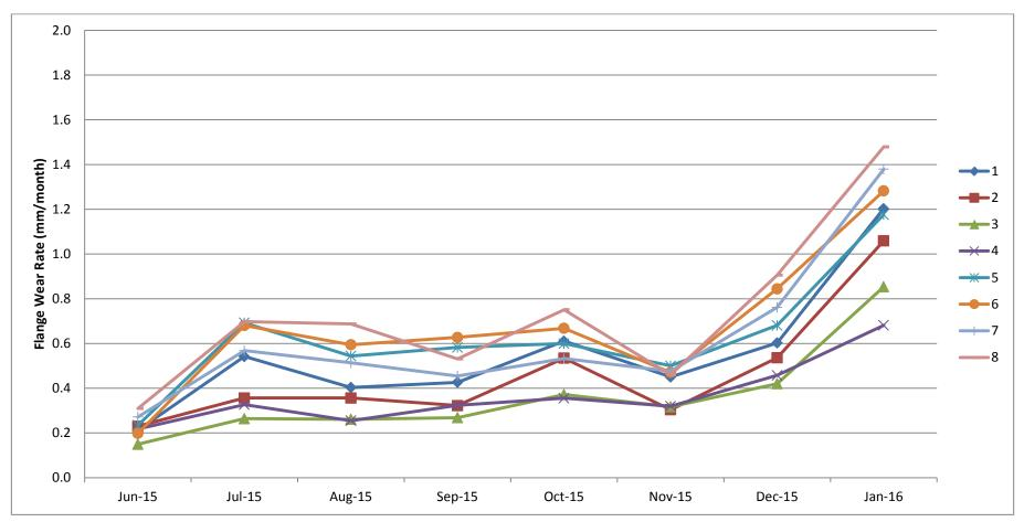
FIGURE C7: FLANGE WEAR RATE MEASUREMENTS FOR ALL WHEELS – 13XX SERIES CAR
