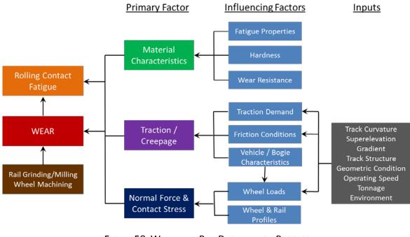
FIGURE 58: WHEEL AND RAIL DEGRADATION PROCESS (MODIFIED FROM [32])
