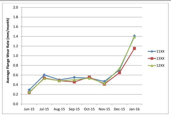
FIGURE 20: VLOCITY FLEET AVERAGE FLANGE WEAR RATE BY CAR SERIES
