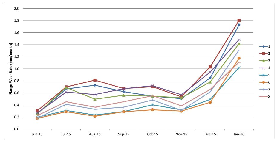
FIGURE C11: FLANGE WEAR RATE MEASUREMENTS FOR ALL WHEELS – 12XX SERIES CAR
