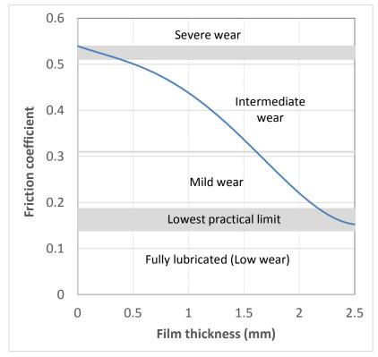
FIGURE 46: GENERAL RELATIONSHIP BETWEEN LUBRICANT FILM THICKNESS, FRICTION COEFFICIENT AND WEAR BEHAVIOUR FOR WHEEL-RAIL CONTACT, BASED ON THE RESULTS OF MCEWEN AND HARVEY [24].
