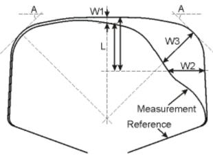
FIGURE 35: RAIL WEAR CALCULATION METHODLOGY
