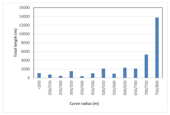
Figure 13: Distribution of Curved Track of R  $\leq$  800 m by Radius and Total Length
