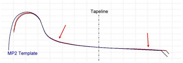
FIGURE 34: EXAMPLE OF ATYPICAL MACHINED WHEEL PROFILE (VS.MP2 PROFILE)
