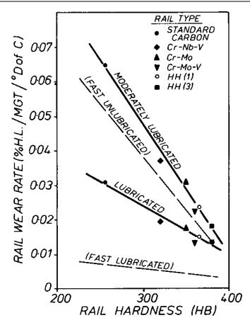
FIGURE 62 GENERAL RELATIONSHIP BETWEEN MATERIAL HARDNESS AND WEAR RATES FOR RAIL MATERIALS FOR VARYING LUBRICATION CONDITIONS [33]
