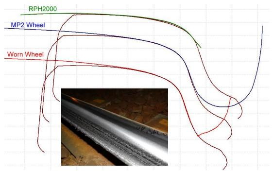
FIGURE 41: HIGH RAIL WEAR (NMFO)
