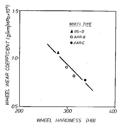
FIGURE 61: GENERAL RELATIONSHIP BETWEEN MATERIAL HARDNESS AND WEAR RATES FOR WHEEL MATERIALS [32]
