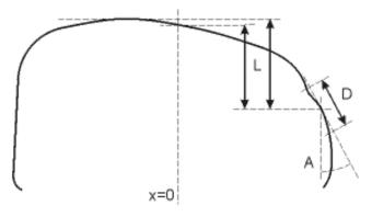
FIGURE 36: RAIL GAUGE ANGLE CALCULATION (AT GAUGE POINT)
