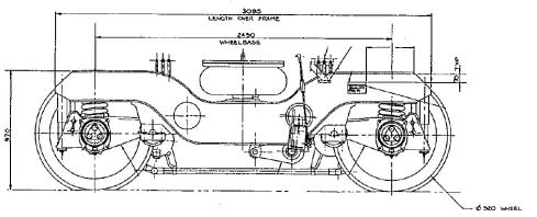
FIGURE 7: SPRINTER BOGIE [11]
