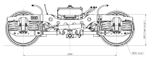
FIGURE 5: VLOCITY BOGIE [8]
