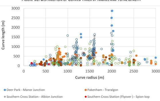
FIGURE 10: DISTRIBUTION OF CURVED TRACK BY RADIUS AND TOTAL LENGTH
