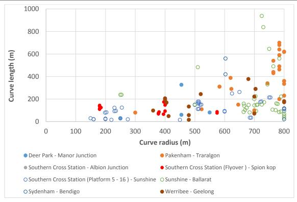
Figure 12: Distribution of Curved Track by Radius and Individual Length, All Curves  $\leq$  800 m Radius
