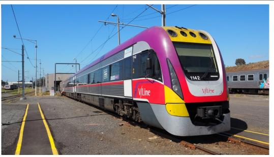
FIGURE 3: VLOCITY 3-CAR DMU
