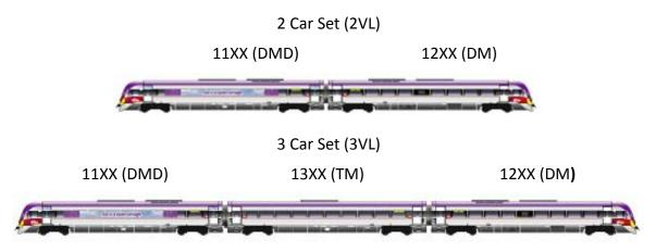
FIGURE 4: VLOCITY TRAINSET CONFIGURATIONS
