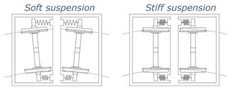
FIGURE 64: BOGIE SUSPENSIONS [35]
