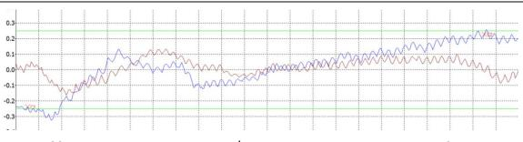
FIGURE 33: VARIATION BETWEEN MEASURED/MACHINED WHEEL PROFILE AND THE MP2 TEMPLATE. [Car 1118, wheels 2 & 7, machined 16/01/2016]
